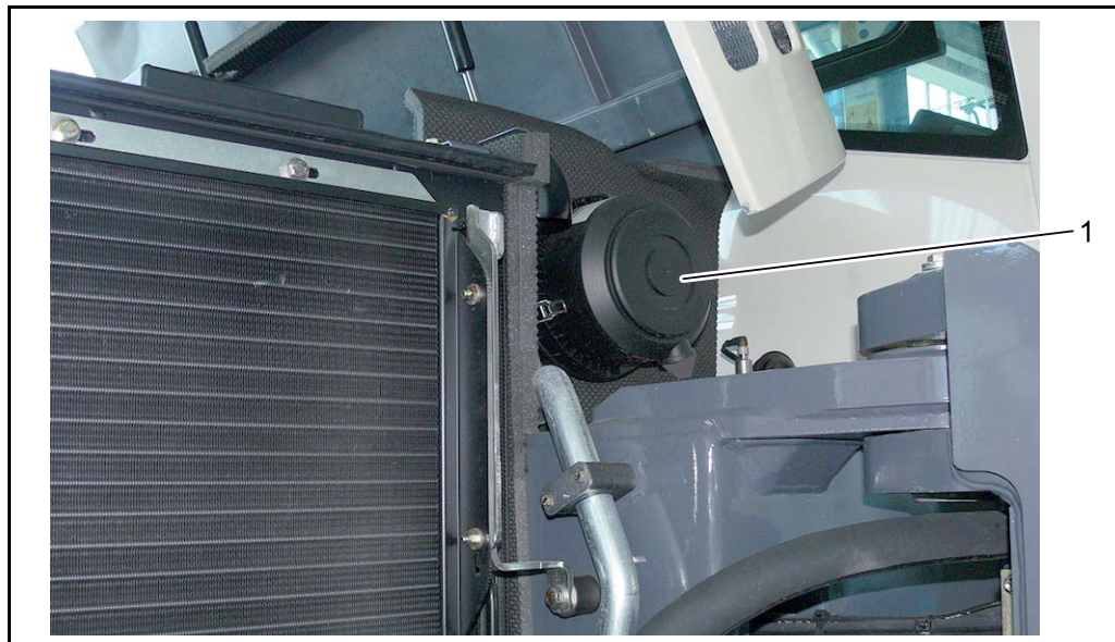
Fig. 6-9 Air filter maintenance
